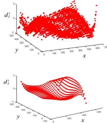
Figure 3. Top: Actual disparity errors, Bottom: Simulated results
