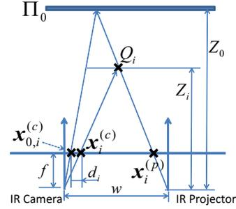
Figure 1. Depth measurement of KINECT
