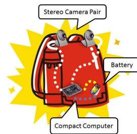
Fig. 2. Components of the WS system. A stereo camera pair is installed on both sides of the top of the backpack, and connected to a compact computer inside the backpack. This system powered by a battery.
